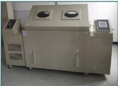
Salt spray test
