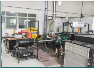
Hybrid system performance test
