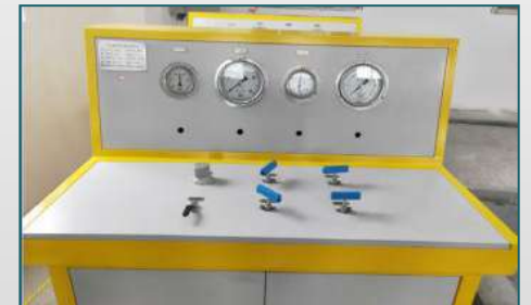
Hydrogen line air tightness test
